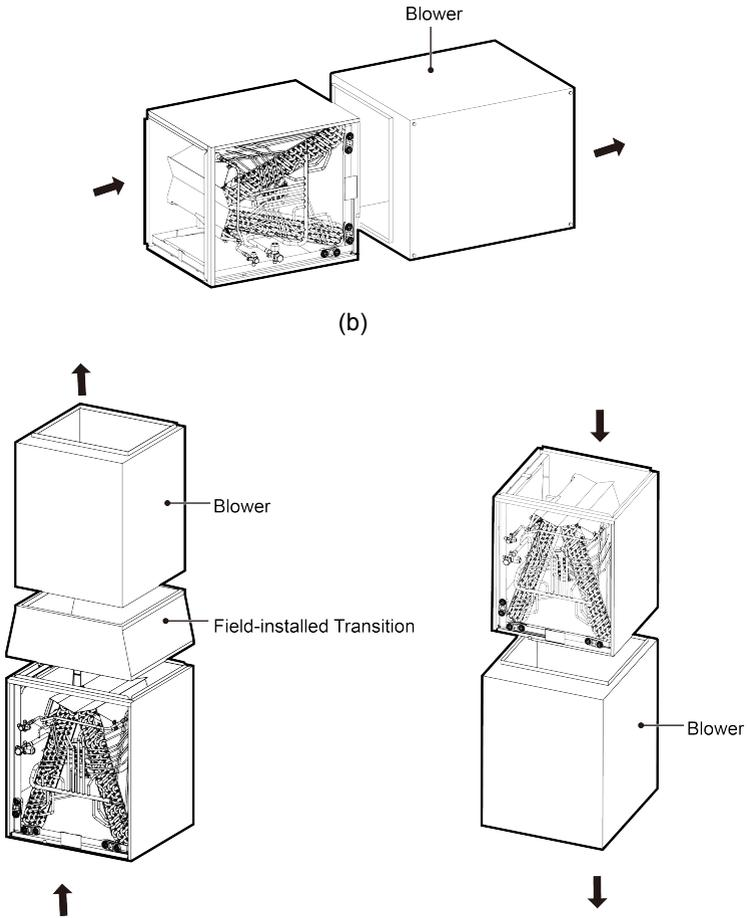
If the air inlet of the blower differs in size from the air outlet of the coil, it may be necessary to install a field-installed transition between the blower and the coil to ensure proper airflow distribution, as depicted in figure (a).
