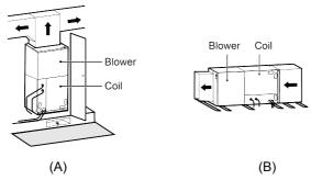
Based upon the actual conditions, Multi-Position A-Coils are factory-installed with both vertical and horizontal drain pans and can be adjusted for either upflow or horizontal pull-through installations. When the coil aligns with the blower, it is prohibited to install an electric heater kit on the side that is close to the coil. The recommended configuration is as illustrated below.
