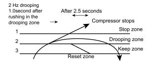
When a "stop current" continues for 2.5 seconds after rushing on the stop zone, the compressor operation stops.
