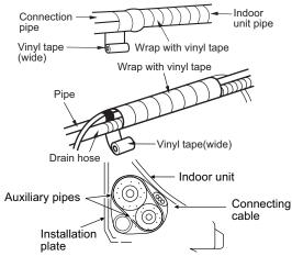
4.Bundle the piping and drain hose together by wrapping them with vinyl tape for enough to cover where they fit into the rear piping housing section.
