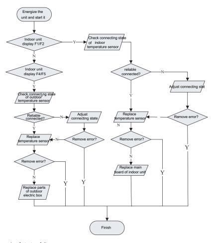
(3) Malfunction diagnosis of startup failure
